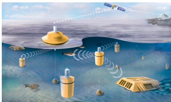
Figure 2.1. Illustration of an underwater sensor network. Illustration courtesy of Underwater Acoustic Network ( http://www.ua-net.eu/ ).
