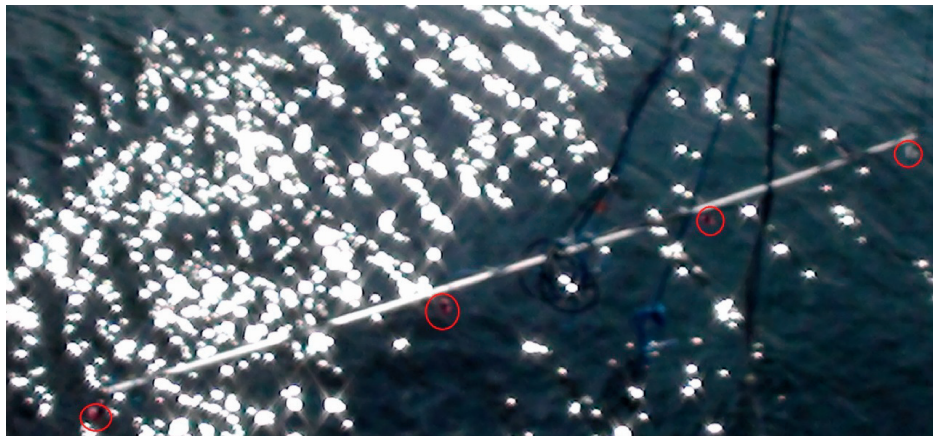
Figure 3.10. HRA of 4 hydrophones. Positions of hydrophones are shown in the red cycles.
