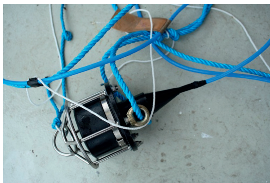
Figure 3.6. High-frequency broadband projector used in experiments.
