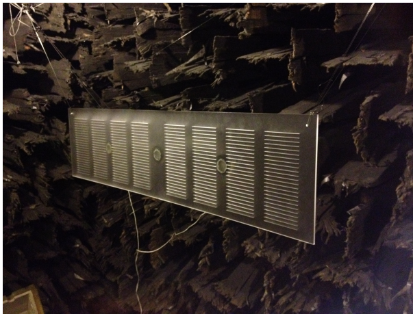
Figure 11: Live picture of the front side of the DML in a anechoic chamber
