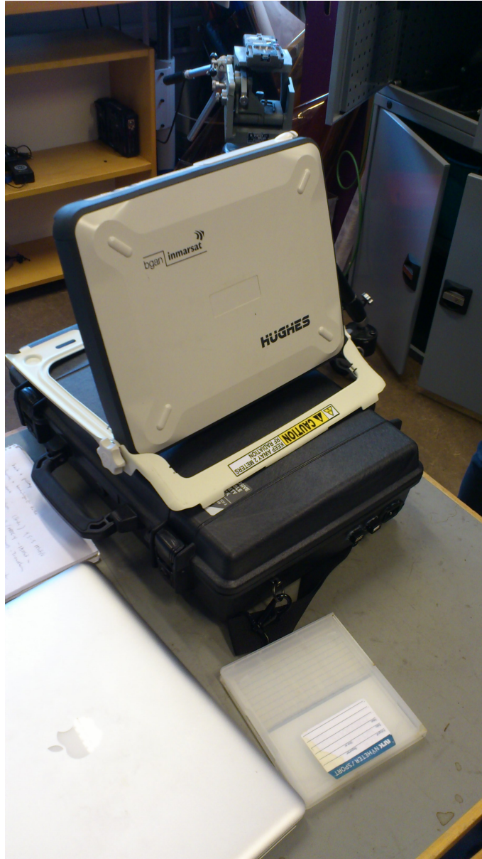
Figure A.3: Photo of a BGAN device. The white "plate" is the satellite transmitter/receiver. Inside the suitcase, there is a laptop which can be connected to the BGAN device. This equipment is easily carried by one person. Photo taken at NRK
