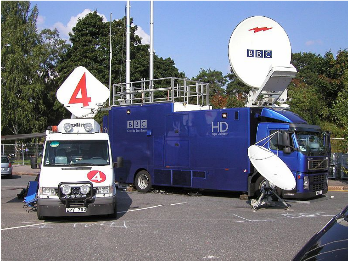
Figure A.2: Photo showing a SNG-truck to the left, and an OB-satellite bus on the right. The OB bus is combined production centre and satellite uplink station. Photo found at wikipedia.org
