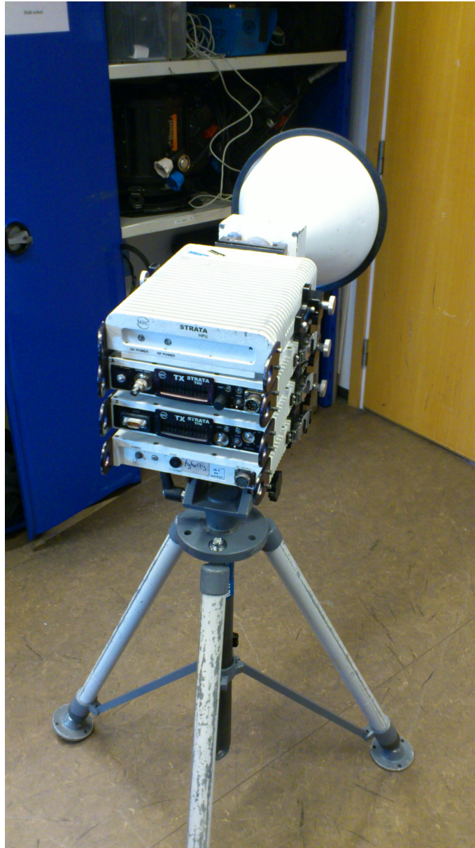
Figure A.4: The microwave solution STRATA used for DENG. The spout is directed towards a receiving antenna up to 70 kilometers away. Photo taken at NRK
