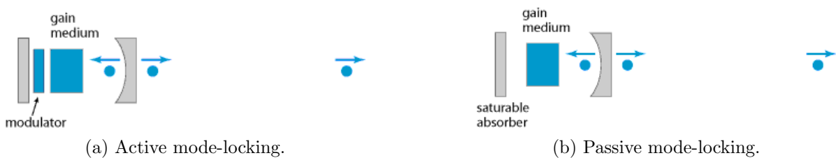
Figure 3.1: Principles of active mode-locking and passive mode-locking [17].
