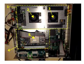
Figure 18: 1. Motherboard Express  $\mu$ ATX. 2-3. Virtex<br/>6 FPGAs. 4.Coretile-Express. 5.The A9 CPU
