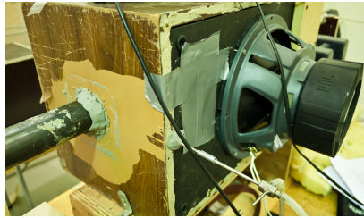
(c) Pipe outlet in a wooden box with an attached loudspeaker transducer.
