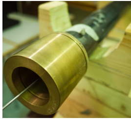
(b) Pipe inlet with cavity and measuring probe,
