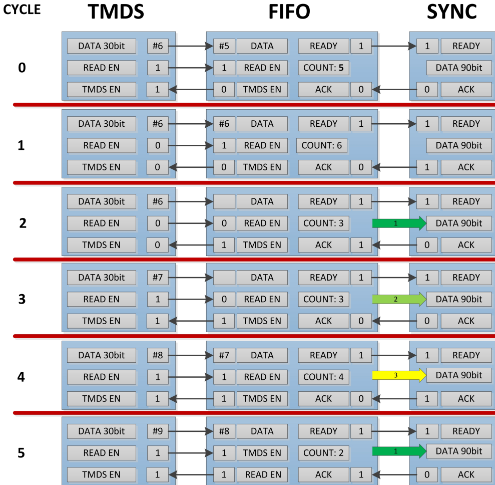
Figure 5.4: Synchronizing the TMDS-modules and the FIFO-module.
