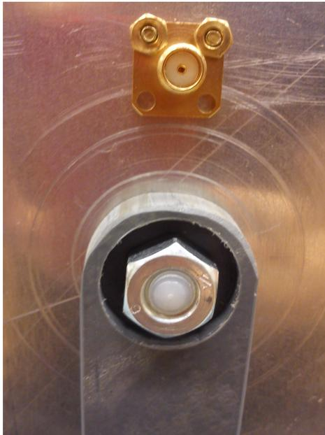
Figure C.3: The back side of one of the ground conductors. In the upper part of the figure is the connector and in the lower part of the figure is the bracket for fastening the antenna on the rotating disc.
