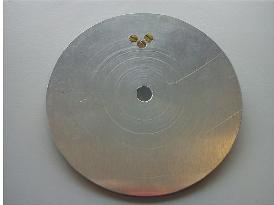
Figure C.4: The flat ground conductor.
