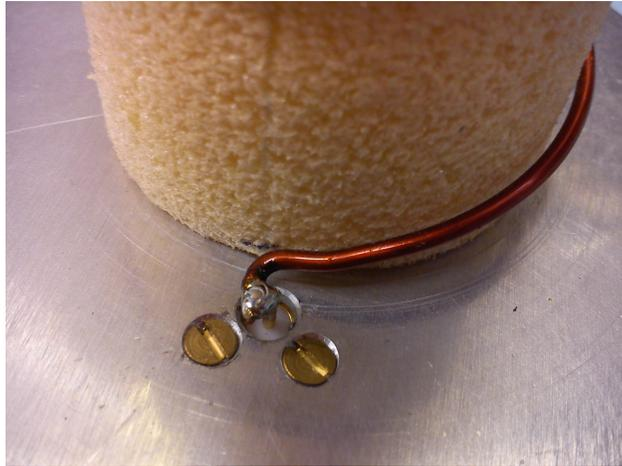
Figure C.2: The connection point between the copper wire and the feed point. The feed is a  $50\ \Omega$  type N connector.
