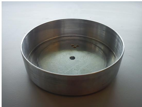
Figure C.5: The cupped ground conductor.
