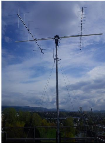
Figure 3.2: The antenna rig at the roof of Electro Block D building at NTNU with two crossed Yagi Uda antennas mounted.
