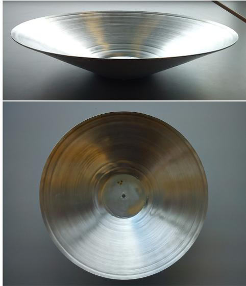
Figure C.6: The truncated cone ground conductor. Top: side view. Bottom: top view.
