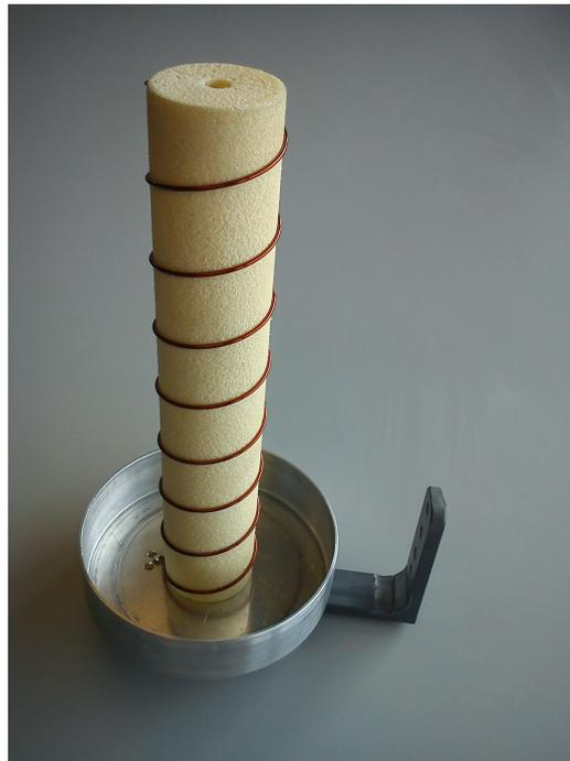
Figure C.1: The helical antenna with the cupped ground conductor. On the right side of the figure is the 90 degree corner angle bracket in plastic for mounting the antenna on the rotating disc.
