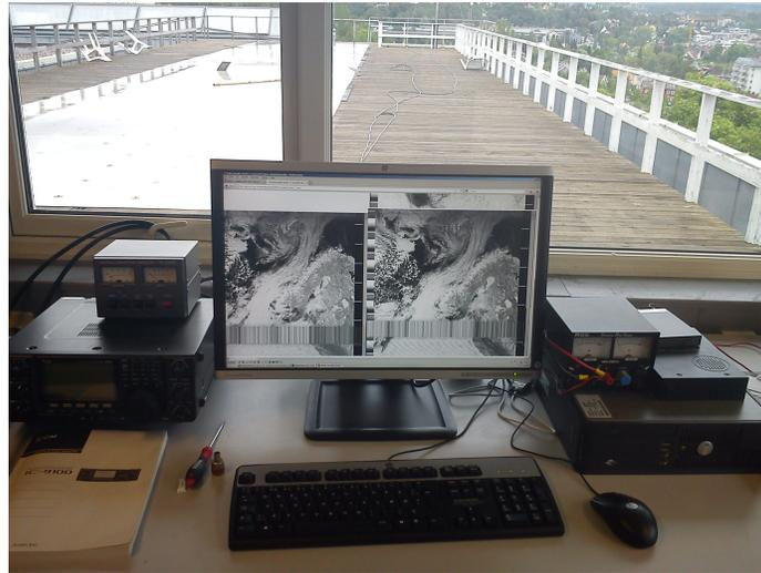
Figure 4.1: To the left: Icom IC-9100 radio and Yaesu G-5500 Elevation-Azimuth Dual Controller. To the right: Yaesu GS-232B Computer Controller with Switching Power Supply, Icom IC-PCR1500 radio for downloading signals from weather satellites and a computer with appropriate software for communication and tracking.
