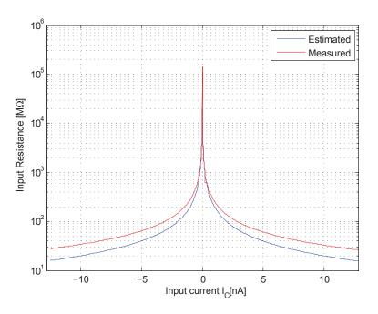
Figure 7.4: Input impedance of the current comparator
