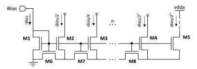
Figure 3.8: Current splitting technique II
