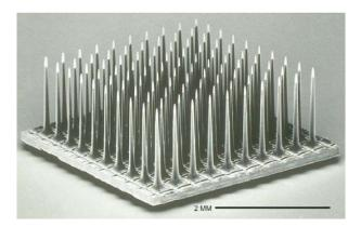
Figure 2.2: The 100-electrode silicon-based Utah Electrode array measuring  $4 \times 4 \times 1.5 mm^3$
