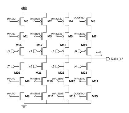
Figure 5.9: Calibration circuit for bit 2-6, though all with different biasvoltages applied
