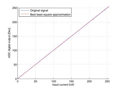
Figure 7.1: Input/output characteristics of the ADC
