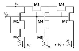
Figure 3.7: Current splitting technique I
