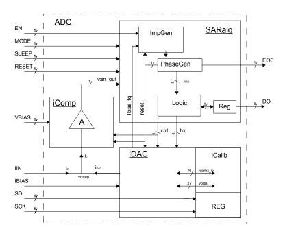
Figure 5.1: System level design for the current mode SAR ADC.
