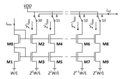
Figure 3.6: Common implementation of a current mode DAC
