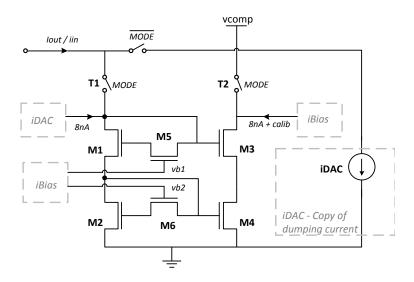
Figure 5.11: Current input/output stage
