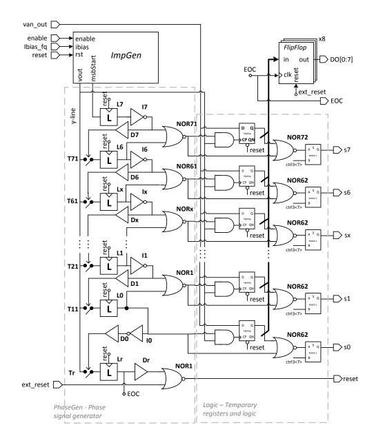
Figure 5.2: Digital circuit used to realize the SAR algorithm and output registers.
