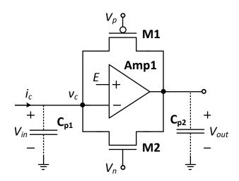
Figure 3.5: Multilevel input impedance current comparator
