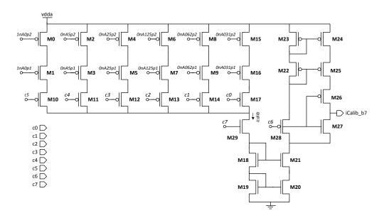
Figure 5.8: Calibration circuit for MSB
