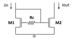
Figure 3.3: SCM with compensation resistor for bandwidth enhancement
