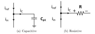
Figure 3.4: Principle of current comparison
