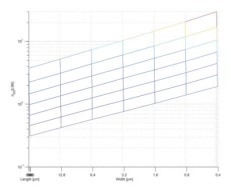
Figure 4.2: SCM Mismatch - Side projection in log-scale
