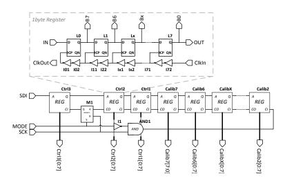
Figure 5.10: calibration register
