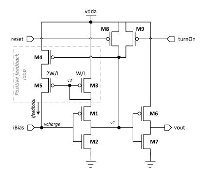
Figure 5.4: Threshold detecting amplifier
