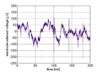
Figure 2.1: Neural recording from a cat motor cortex using Utah Electrode Array and CMOS amplifier.
