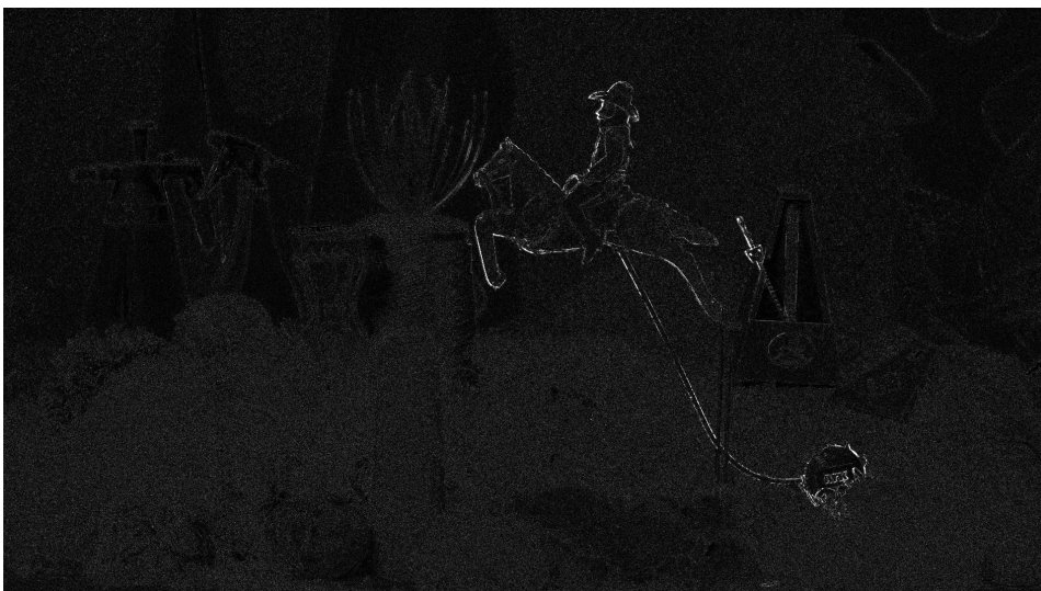
Figure D.16: Estimation error of 115 of frame 1 of Horse sequence. White indicates estimation error. Optical flow vector field with a resolution of 1920x1080 and quarter pixel accuracy.
