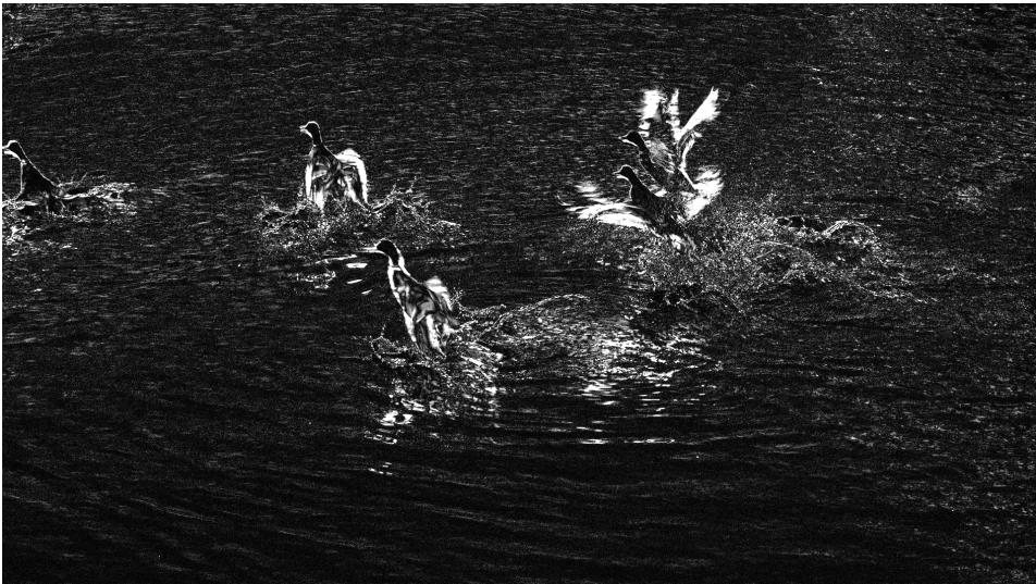
Figure D.6: Estimation error of frame 13077 of DuckTakeOff (Ducks) sequence. White indicates estimation error. Optical flow vector field with a resolution of 1920 \times 1080 and quarter pixel accuracy.
