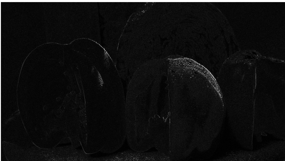
Figure D.14: Estimation error of frame 13 of Vegies sequence. White indicates estimation error. Optical flow vector field with a resolution of 1920 \times 1080 and quarter pixel accuracy.
