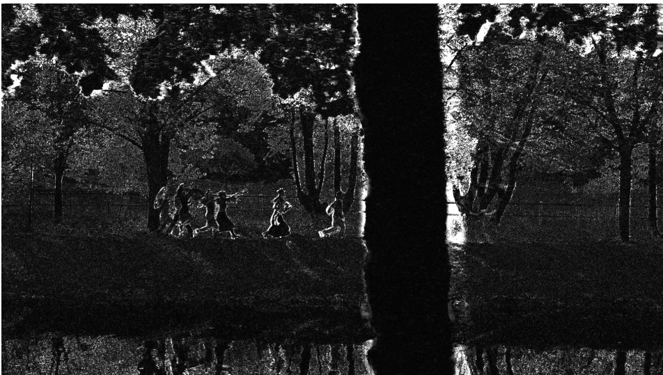
Figure D.12: Estimation error of frame 15739 of Parkjoy sequence. White indicates estimation error. Optical flow vector field with a resolution of 1920x1080 and quarter pixel accuracy.
