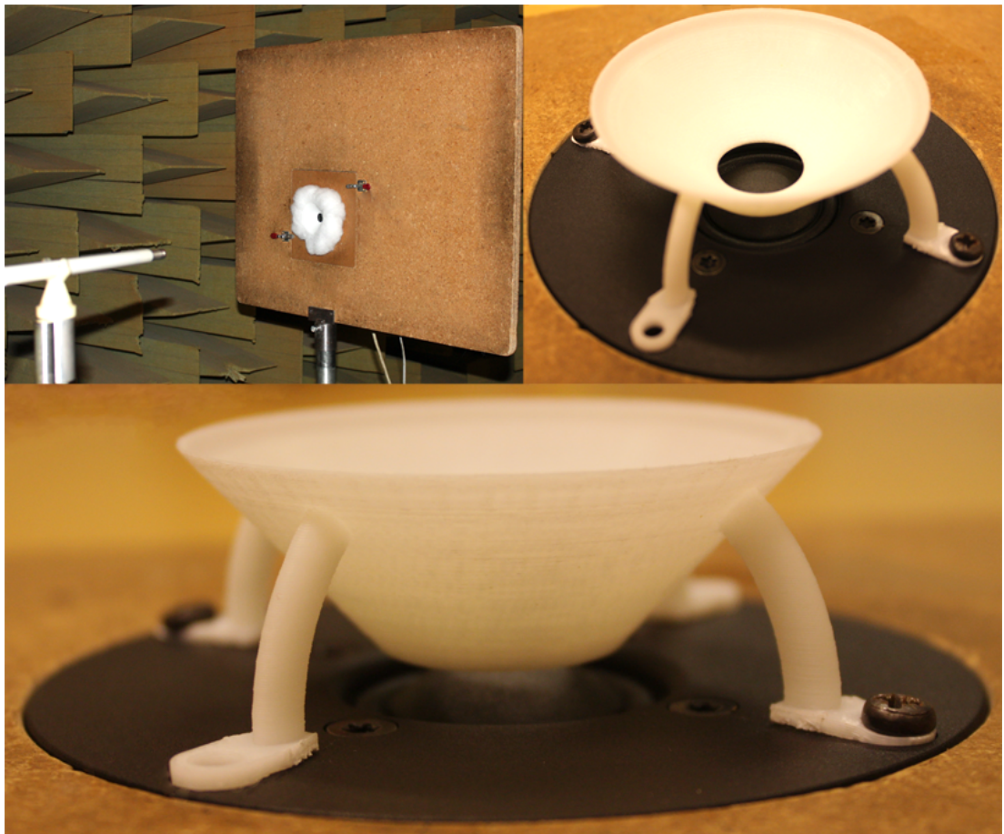
Figure 3.16: Upper left: Prototype measurement setup (with damping) Upper right & bottom: Prototype waveguide mounted on tweeter.
