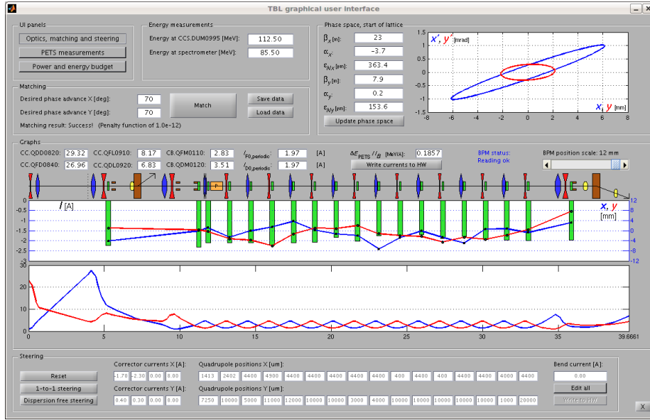
Figure 4.1: The GUI screen for optics, matching and steering. A larger version of the figure is provided in Appendix D.
