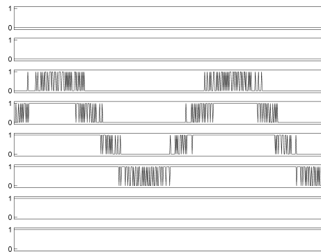
Figure 53: Switching sequence for each element in a 3-bit DSM DAC
