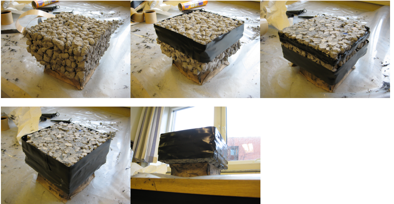
Figure 26: Construction of flow method samples
