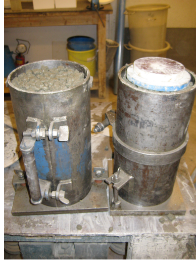
(b) Filled compacted forms and shim plate
