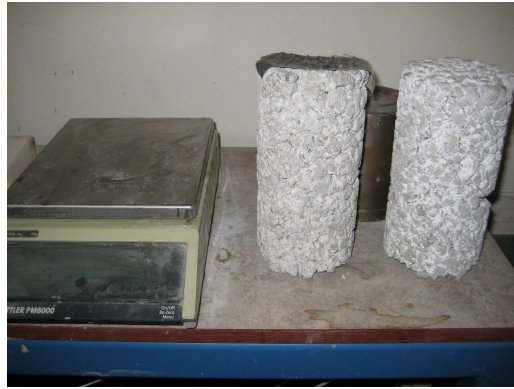
(b) weighing of dry specimen
