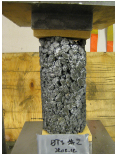
Figure 24: Uneven test surface
