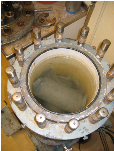
(f) Specimen placed in pressure chamber
