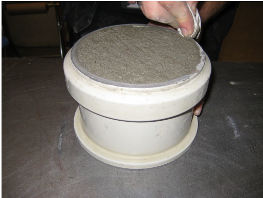
Figure 9: Mortar in 1 liter container
