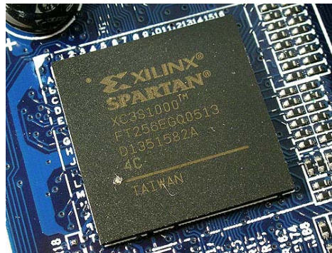
Figure 19. Picture shows a Xilinx Spartan 3, XC3S1000-4FT256C (17x17mm).
