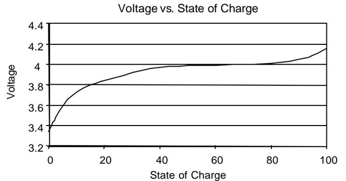
Figure 5. Open Cell Voltage of Lithium Polymer Battery
