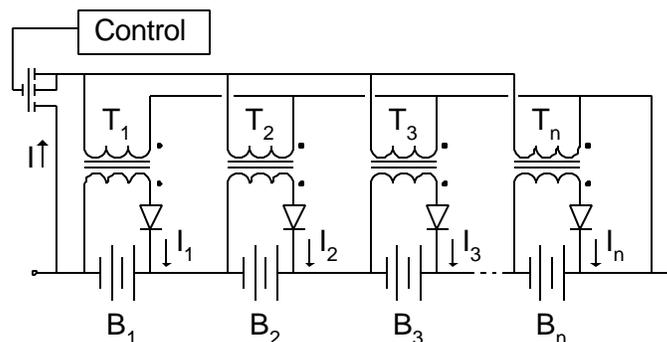
Figure 8. Multiple Transformer
