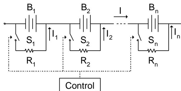
Figure 9. Dissipative Method
