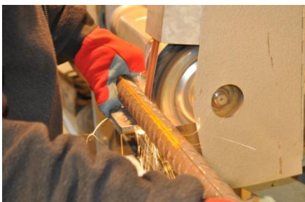
Figur 13: Armeringen blir grovslipt
