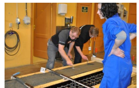
Figur 36: Betong uten fiber bearbeides
