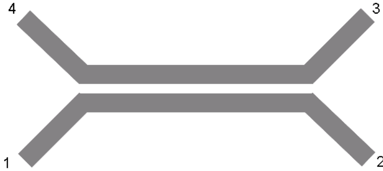
Figure 2.4: Coupled-line directional coupler
