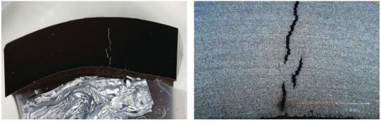
(a) Internal crack
