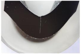
(a) Visible crack through 75 % of the thickness
