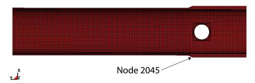
Figure 7.8: Springback simulation constrained against rigid body motion at node 2045.
