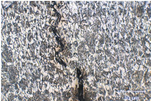
(c) Deformation near crack tip
