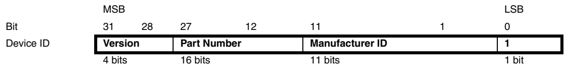
Figure 4-18. The format of the Device Identification Register
