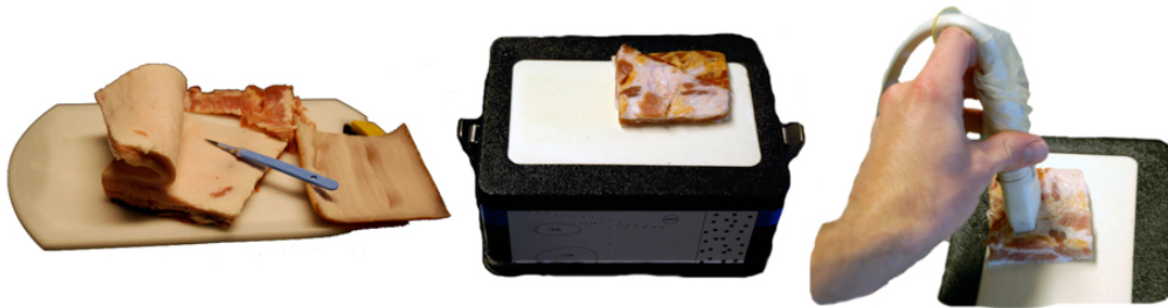
Figure 6.4: Imaging on phantom with bacon as reverberation model
