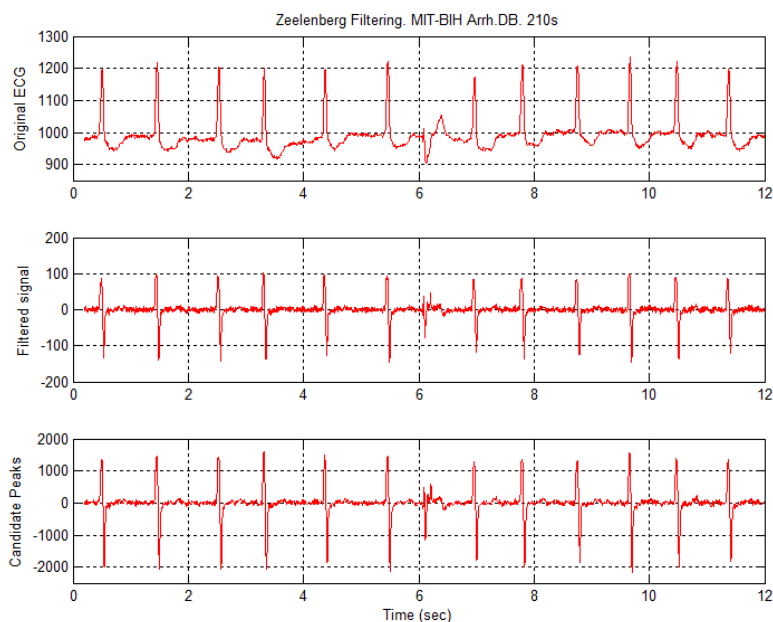
Figure 6.9. Zeelenberg filtering stage applied to an excerpt of record 210 of MIT-BIH Arrhythmia Database
