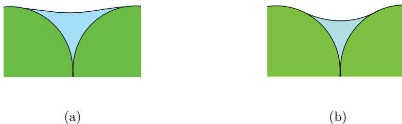
Figure 2.14: Change in water surface deformation between two spheres partially immersed in a water film with a change in film thickness as the water evaporates.
