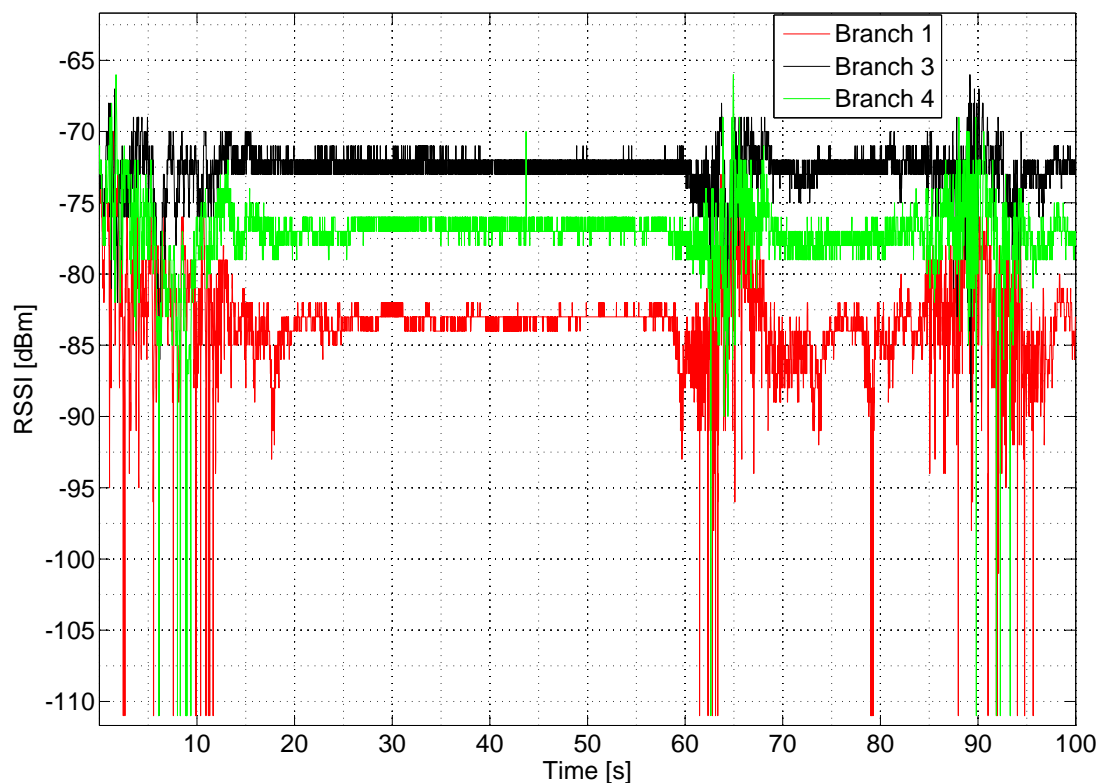
Figure 6.8: Static RSSI measurements for the entire lapse of transmission
