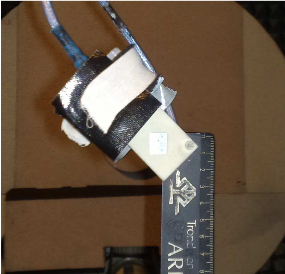
Figure 9.25: Picture of the measurements setup for H-plane measurements. The SMA-to-microstrip launch is covered with absorbers.
