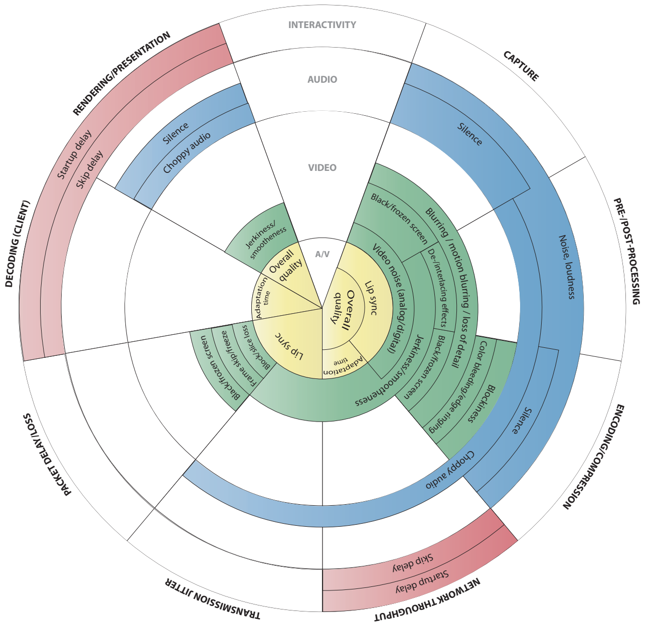
Figure 2.7: Overview of where degradation to video stream may occur in the service delivery, based on [32, 62, 57, 67, 68, 69].
