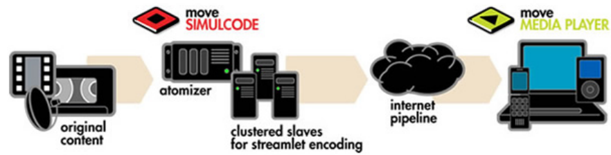
Figure 3.2: An overview of the Move Simulcode process [9].
