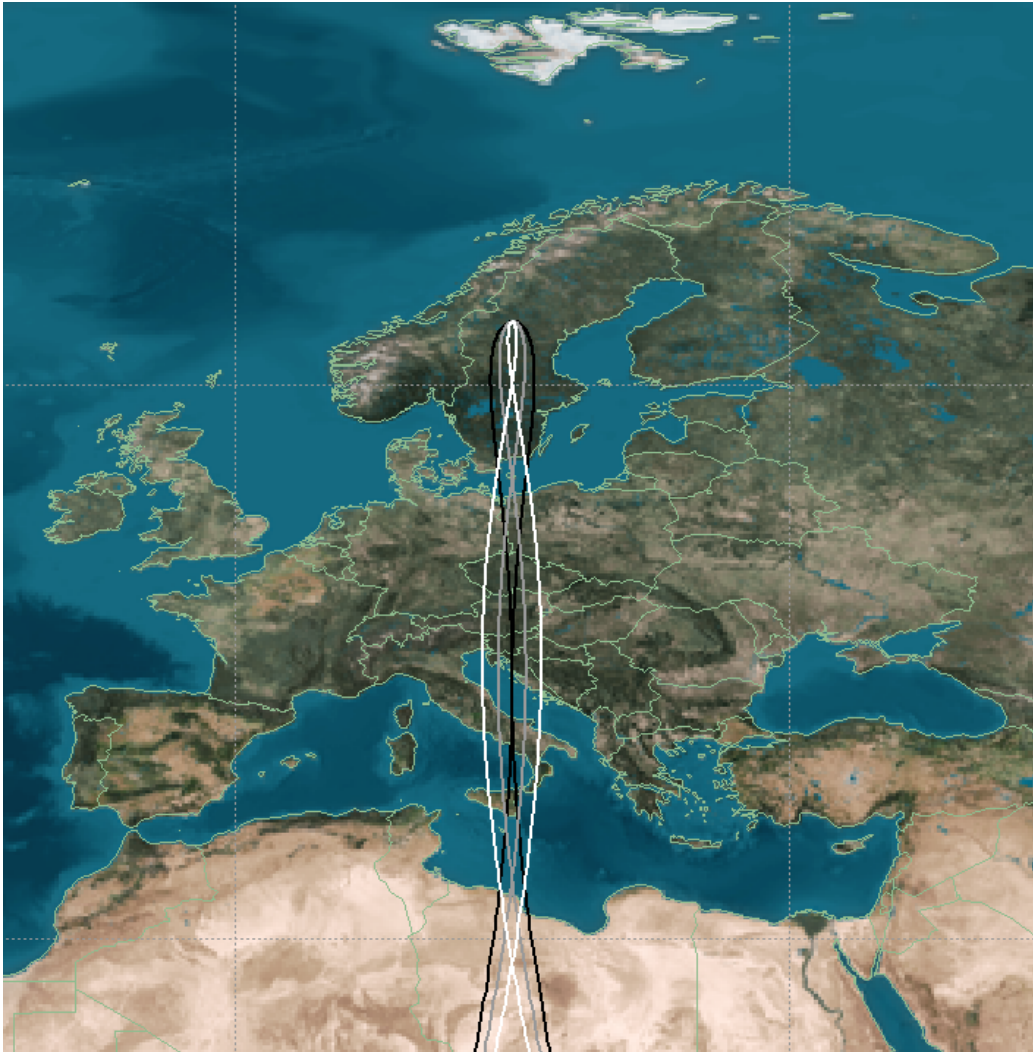
FIGURE 9: The ground track of three Molniya orbits with different eccentricity. When the most northern intersection point is used for handover a satellite will spend eight hours in the black loop, six in the grey and four in the white. The ground track intersection point is placed fairly arbitrarily at 15^\circ east.
