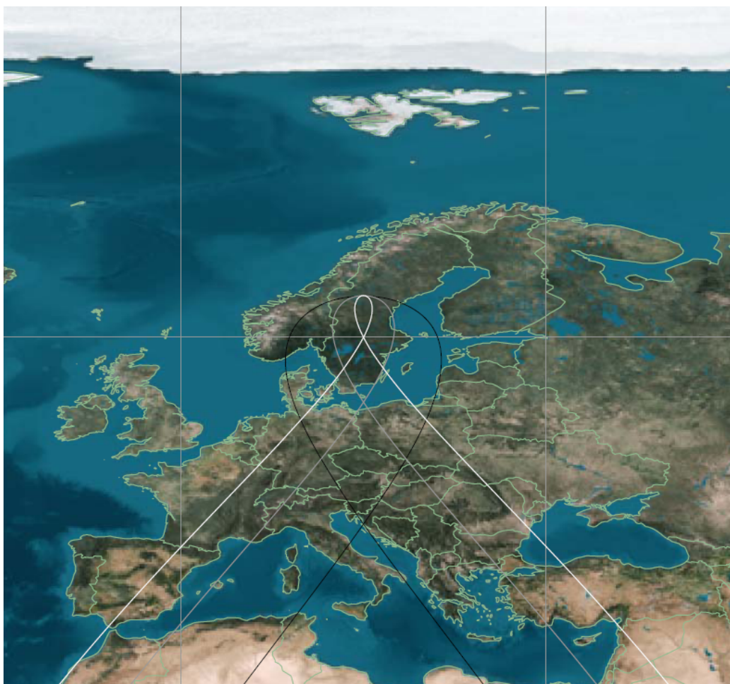
FIGURE 7: The ground track of three Tundra orbits with different eccentricity. A satellite will spend eight hours in the black loop, six in the grey and four in the white. The ground track intersection point is placed fairly arbitrarily at 15^\circ east.
