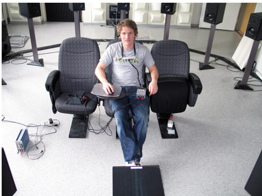
Figure 7.2: Rhyme test showing a test person sitting centered between speakers with the microphone array worn on his chest.
