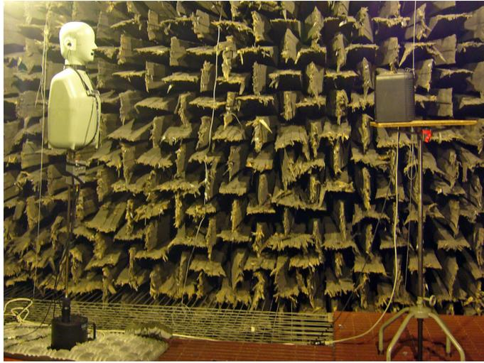
Figure 6.2: HATS and speaker seen in anechoic chamber
