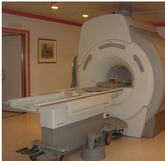
Figure 3.7: The 1.5 T clinical MR scanner used in the experiments. The mouse coil is in the iso-center of the MR scanner.
