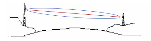
The concept of Fresnel's area is really important when we are dealing with electromagnetic waves. As most of the energy is concentrated on this area this part should not be obstructed by an obstacle, such as a building or a forest. The introduction of an object will introduce some reflection and diffraction effects, which will disturb our received signal.
