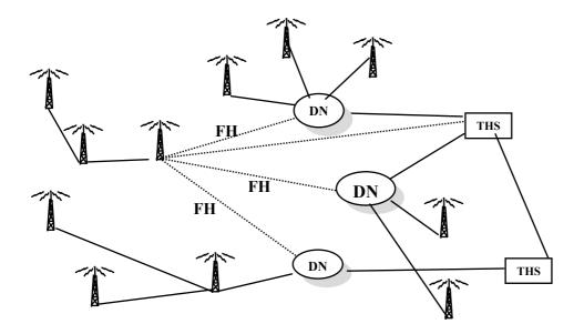
The DN is linked to a BSC (or sometimes another DN) with the help of an electromagnetic wave with a small frequency (13 or 18 GHz) and an important capacity (16\*2, 20\*2, or 40\*2
