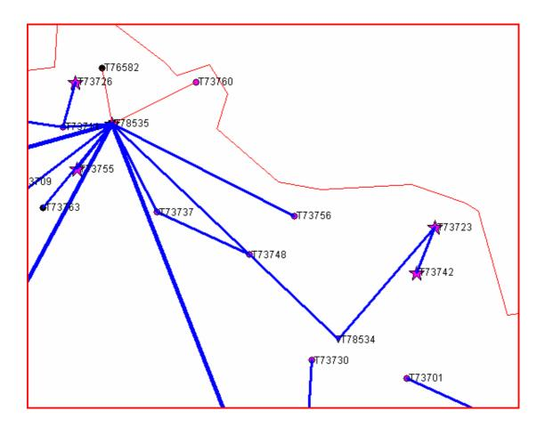
When we study the area, we see than after the leaving of the T78534, 2 sites will no more be connected to the transmission network: the sites number T73742 and T73723. We have to find a new distant site for these 2 sites.
