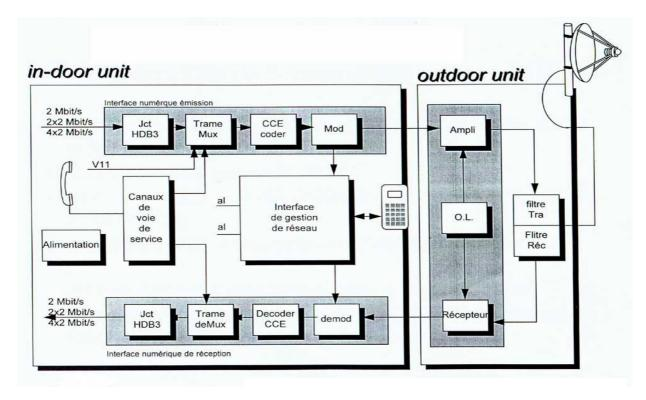
Most of the time, the ODU is attached to the antenna's back. As for the IDU, it is installed in a special shelter. In the case of nodal sites (DN, BSC or MSC) a lot of IDU are present in the shelter(s).
