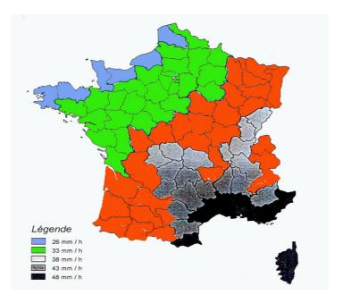
To represent the attenuation due to the rain, the country has been divided in different categories, according to the pluviometry of the area, and more precisely the quantity of rain per hour for the 53 worst minutes in the year.
