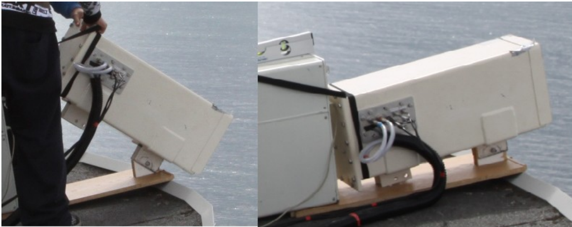
Figure 49: Wood made structure to handle the laser
