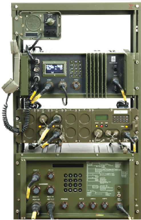
Rack with RL532A, Bulk Encryption Unit CD510 and Multimedia Switch CPX300
