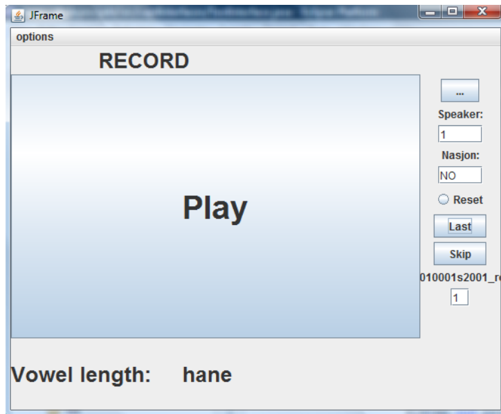
Figure 3.1: The recording interface used in this work. The user is only supposed to click on the button marked 'Play' which changes into 'Record', then back to 'Play' again, and so on. The rest of the buttons are for the recording supervisor.
