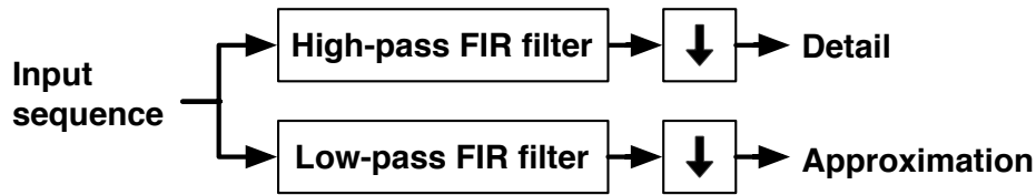
Figure 3.2: One dimensional Wavelet Transform computed with filter bank.
