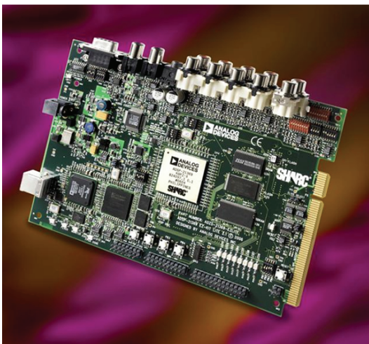
Figure 10.1. ADSP-21369 SHARC EZ-KIT Lite Evaluation Kit.
