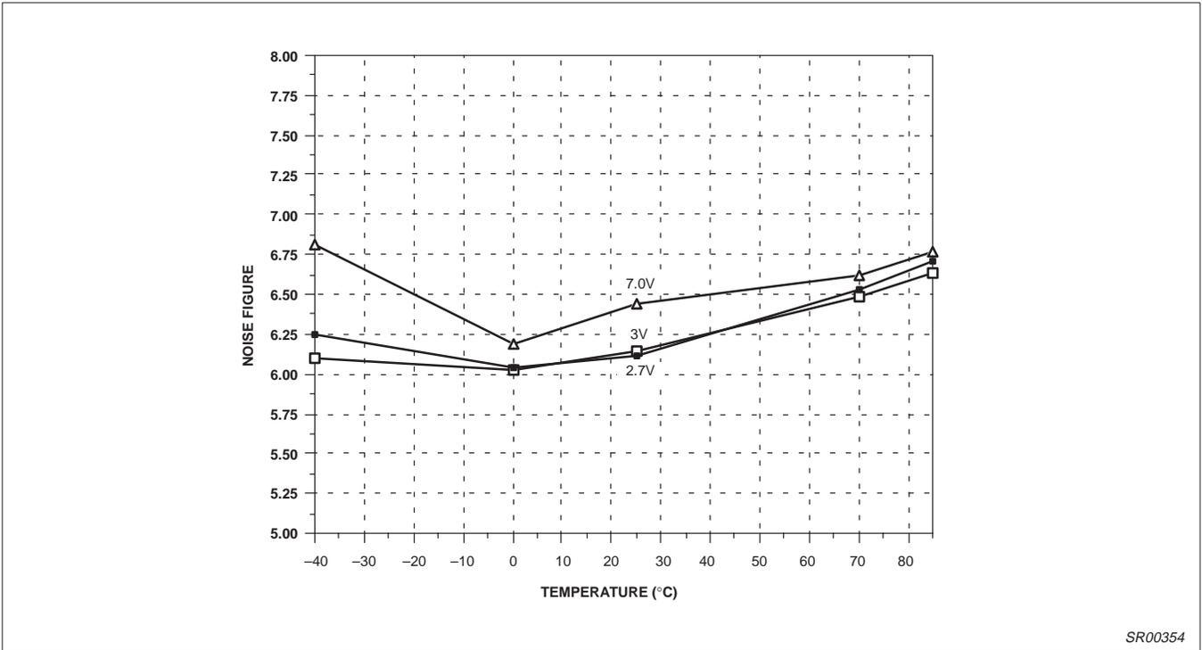
Figure 8. Mixer Noise Figure vs Supply Voltage
