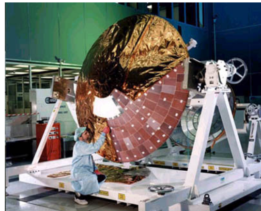
Figure 3: MLI blankets on Huygens' front shield.
