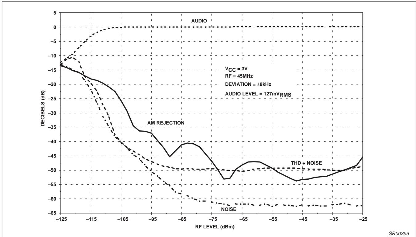
Figure 13. Sensitivity vs RF Level (Temperature 85°C)
