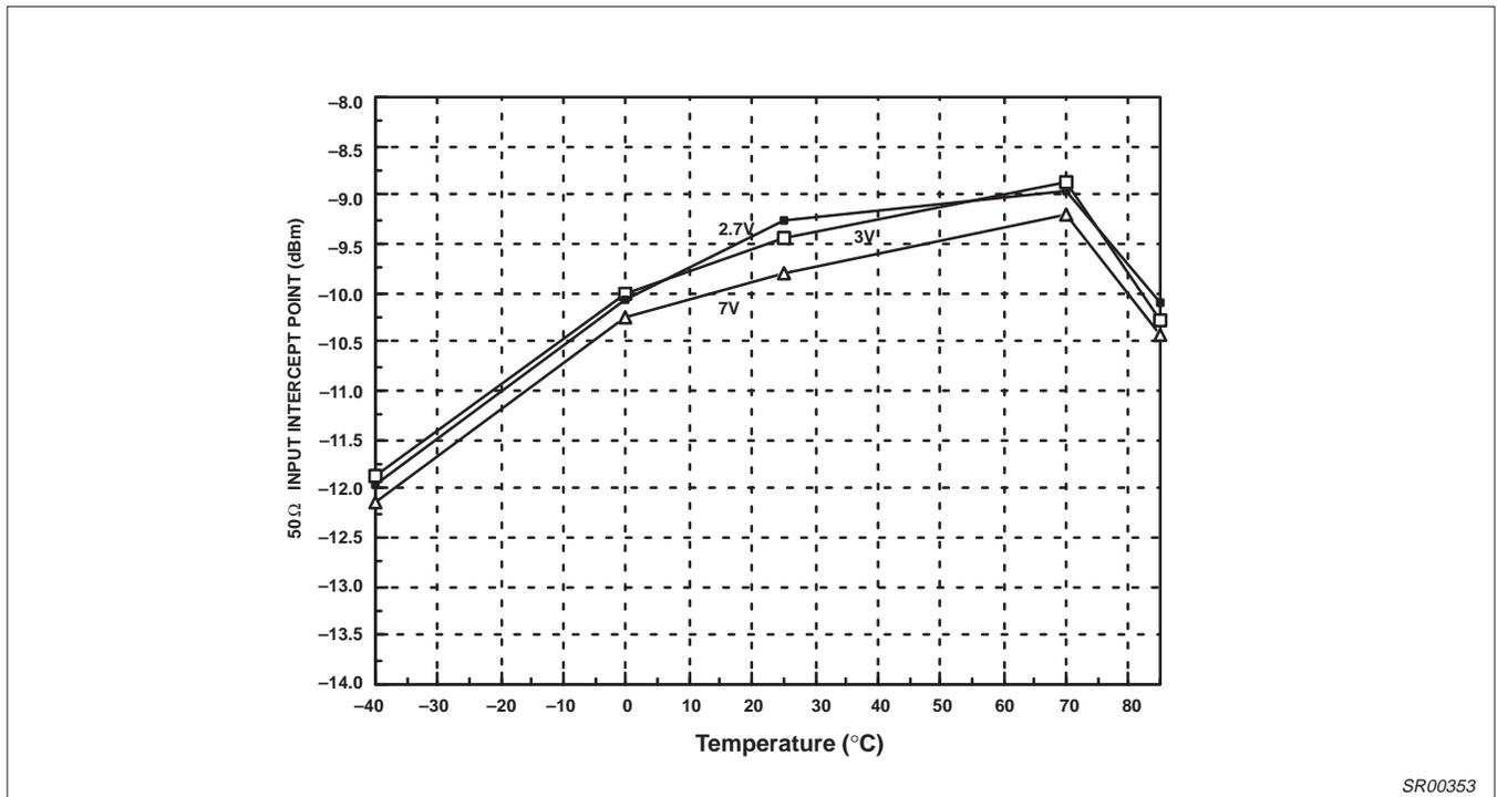
Figure 7. Third Order Intercept Point vs Supply Voltage
