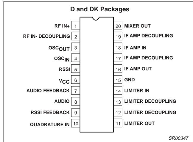
Figure 1. Pin Configuration
