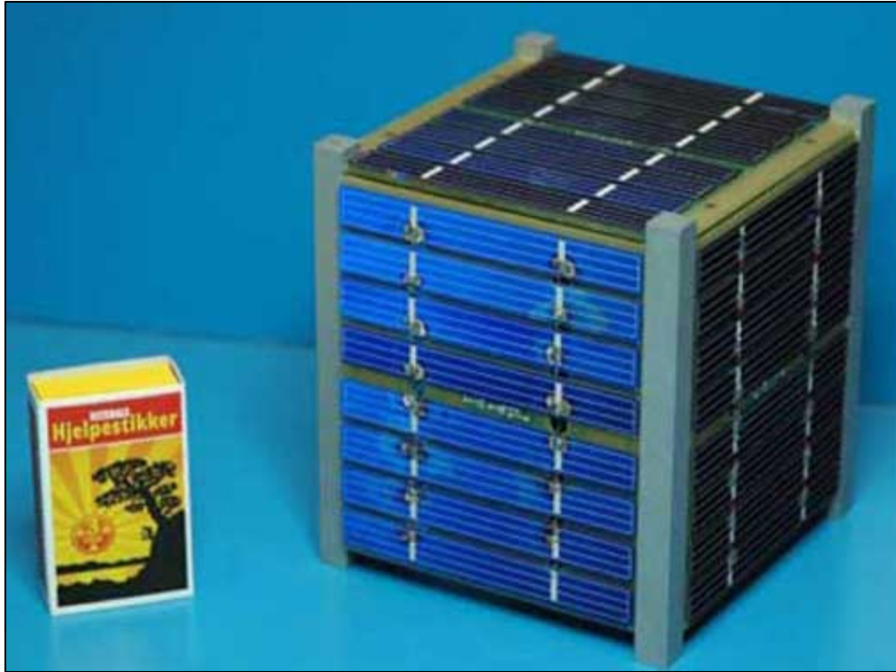
Figure 4: A CubeSat where the exterior walls are covered with solar cells.
