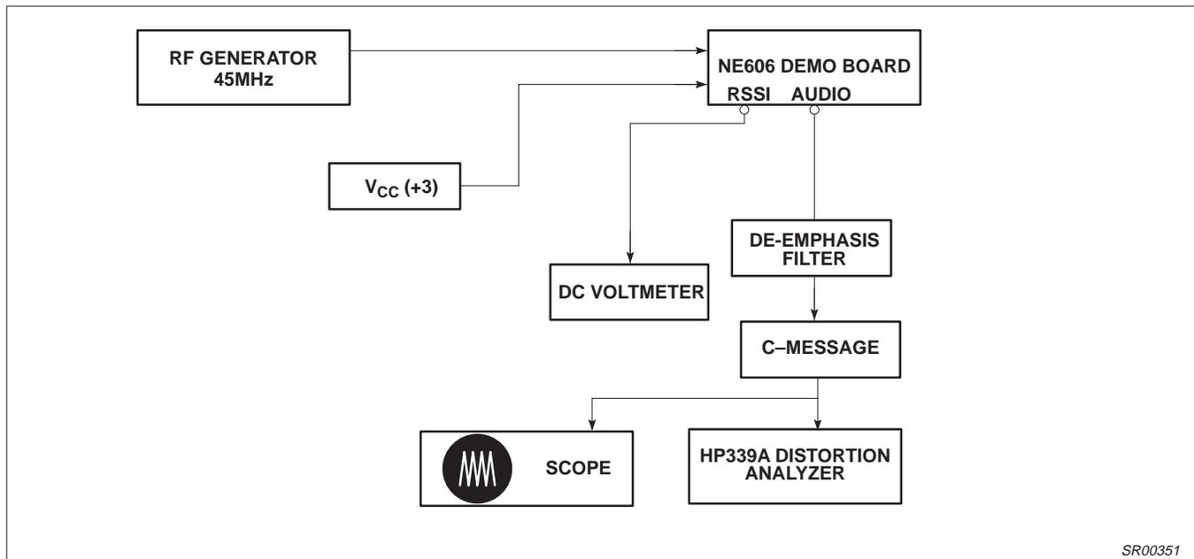
Figure 5. SA606 Application Circuit Test Set Up
