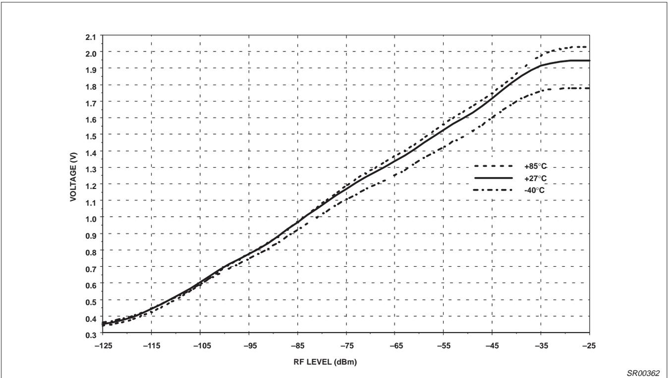
Figure 16. RSSI vs RF Level and Temperature - V<sub>CC</sub> = 3V
