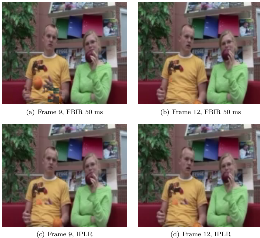
Figure 4.3: Visual artifacts and recovery behaviour. Three bottom GOBs of frame 8 is lost. Conversation, 144 kbit/s.
