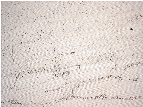
Figure 11.6: Surface of a silicon bar after polishing seen through a light microscope. Some pointwise defects from the grinding process are still left.
