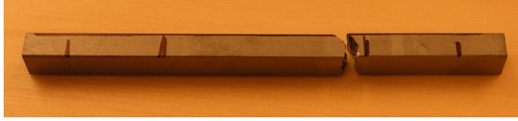
Figure 11.9: Example of discarded sample, in which fracture took place too close from an inner roller (whose position is approximated by a vertical bar).
