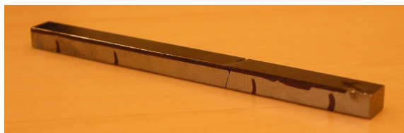
Figure 11.4: Etched specimen marked and tested. The vertical bars indicate the approximate position of the inner and external rollers and allow to validate the test.
