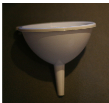
Figure 2.7 Kitchen funnel used for BIAS measurements in figures 3.11 and 3.12. The funnel has a diameter of about 8 cm at the widest opening, and 8 mm at the narrow end.
