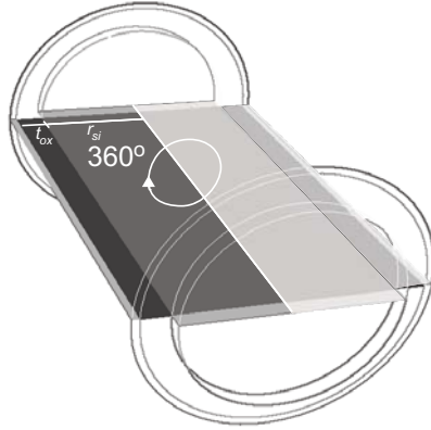
Figure 6.3: Radial cross-section of the GAA MOSFET. This surface must be rotated 360^\circ about the central axis to cover the cylindrical volume.
