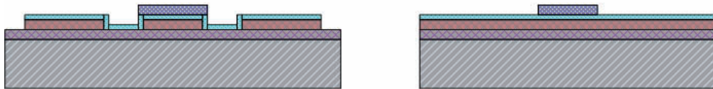
10) Expose the resist in automatic aligner and develop in standard developer. Hardbake the resist in oven.
