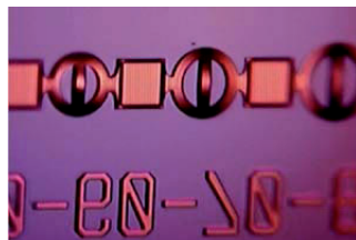
Figure 2: Optical images of buckled guckel ring and cantilever sputtered at 10 mTorr and 500 watt
