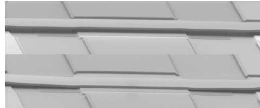
Fig. 3 SEM images of the fabricated switch in its idle (top) and actuated (bottom) states.
