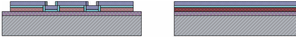
9) Priming and HIPR 6512 resist coating in automatic coater. The thickness is 1.5 \mu\text{m} .
