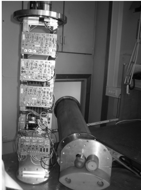
Figure 4.2: A photography of the open cylinder containing the electronics. The transducers are shown to the right. The 1 MHz transducer is the smallest one to the left, the 710 kHz is to the right and the 200 kHz is at the bottom.
