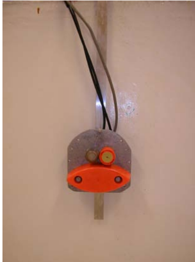
Figure 5.2: A photography of the transducers mounted on the wall of the water tank. The upper left transducer is the 1 MHz transducer produced at the Department of Electronics and Telecommunications at NTNU. The upper right is the 710 kHz and the lower is the 200 kHz transducer produced by Simrad AS.
