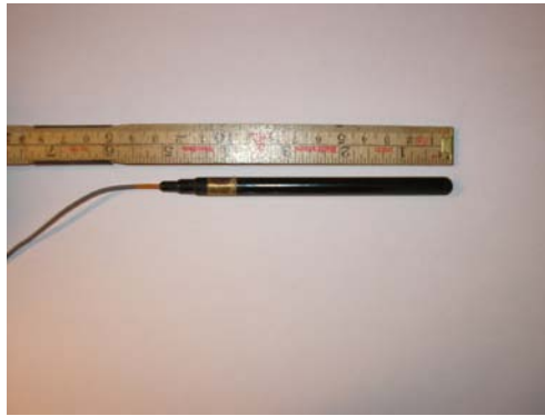
Figure 5.1: The Model ITC-6128 TM hydrophone from International Transducer Corporation used in the calibration measurements.
