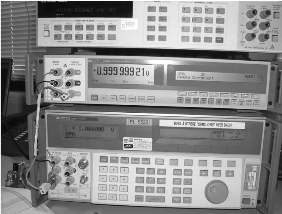
Fig. 4.5: Image of the instrument setup. Two multimeters were transported from Kjeller to Stavanger, then used to calibrate an electrical calibrator, after which they were returned to Kjeller for recalibration.
