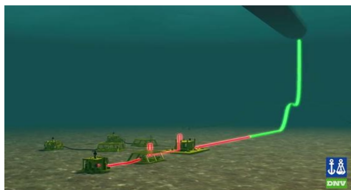
Fig. 5-2: Sub-sea system pipeline
