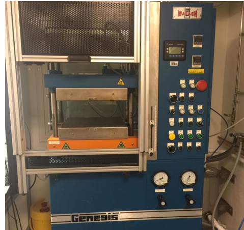
(b) Mechanical press with temperature regulated plates for SIR molding.
