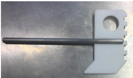
(a) For the mixing of the silicon rubber components a PTFE stirrer is used.
