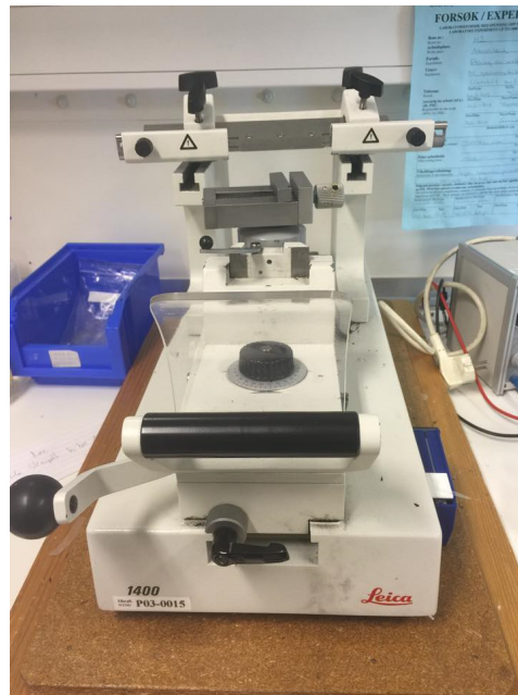
Figure 5.1: Preparation of XLPE samples. A table-knife is used for the fine cutting of the specimens before the surface preparation.
