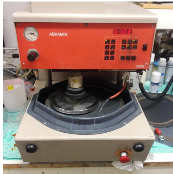
Figure 5.6: The STRUERS Abramin rotating grinding machine while in use. The samples are being grinded while water is flowing.
