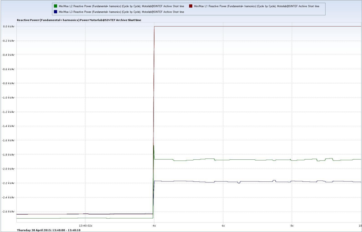
Figure A-13: Experiment 2. Start open conductor fault event.
