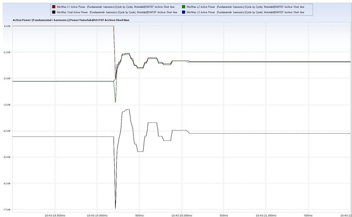
Figure A-16: End open conductor fault experiment. Oscillation period t \approx 300 ms. Peak RMS value 7 kW in total. The faulty phase is reconnected and the oscillations are damped out after one second.
