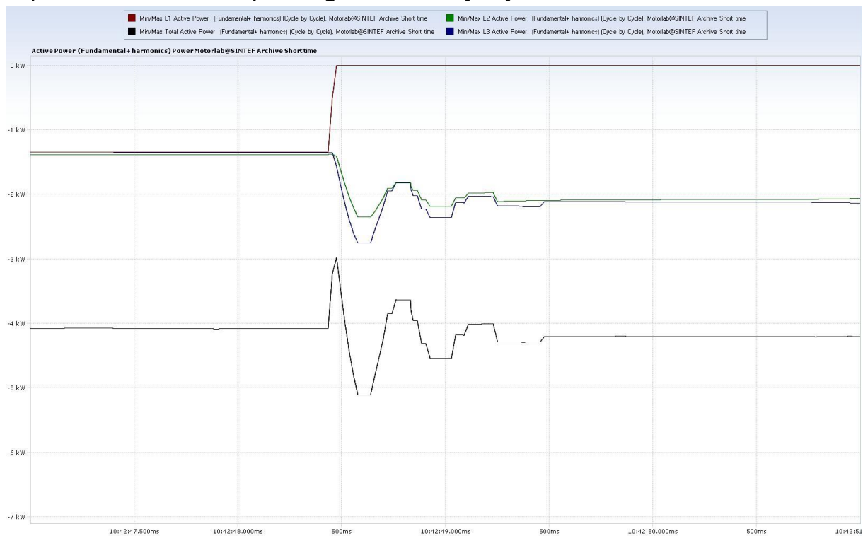
Figure A-15: Start open conductor fault experiment. Oscillation period t \approx 300 ms. Phase powers L2 and L3 changes from 1,5 kW to 2 kW during the fault. The oscillations are damped out after one second.
