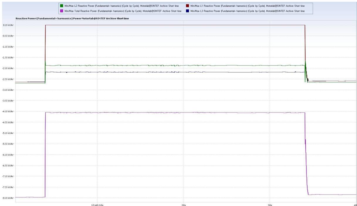
Figure 51: Total- and reactive phase powers during the open conductor fault experiment.
