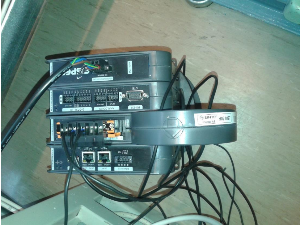
Figure 44: The Elspec Blackbox installed in laboratory.
