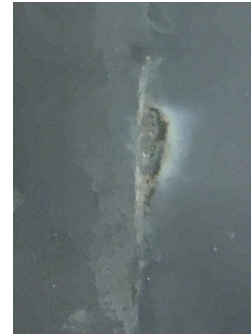
Figure 170. Closer look at a point where a heat generation have made a mark on the stress control tube.
