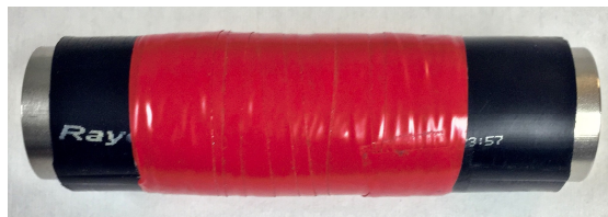
Figure 167. Wet test object with plastic foil and PVC insulation tape.
