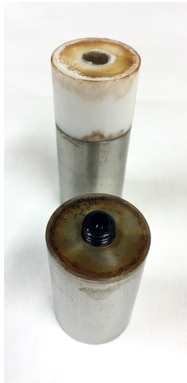
Figure 171. Metal electrodes and PTFE rod from the wet test object. Rust is observed at each electrode.
