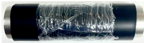
Figure 168. Wet test object wrapped in plastic foil.
