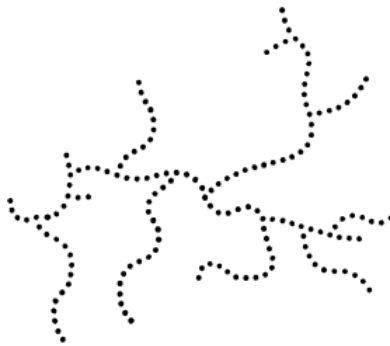
Figure 2.1: Polyethylene chain with side branches [5, p. 9].
