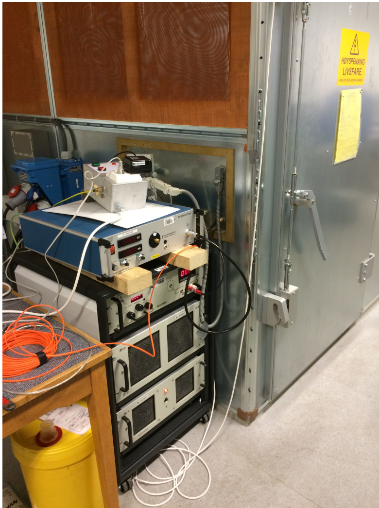
Figure A.1: Picture of the experimental setup from outside the faraday cage with the voltage sources, top: DC source, bottom: Behlman
