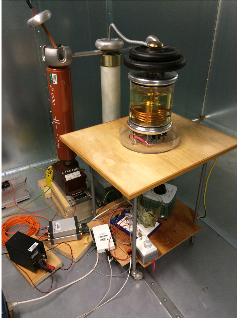
Figure A.2: Picture of the experimental setup inside the faraday cage with the testcell in the center
